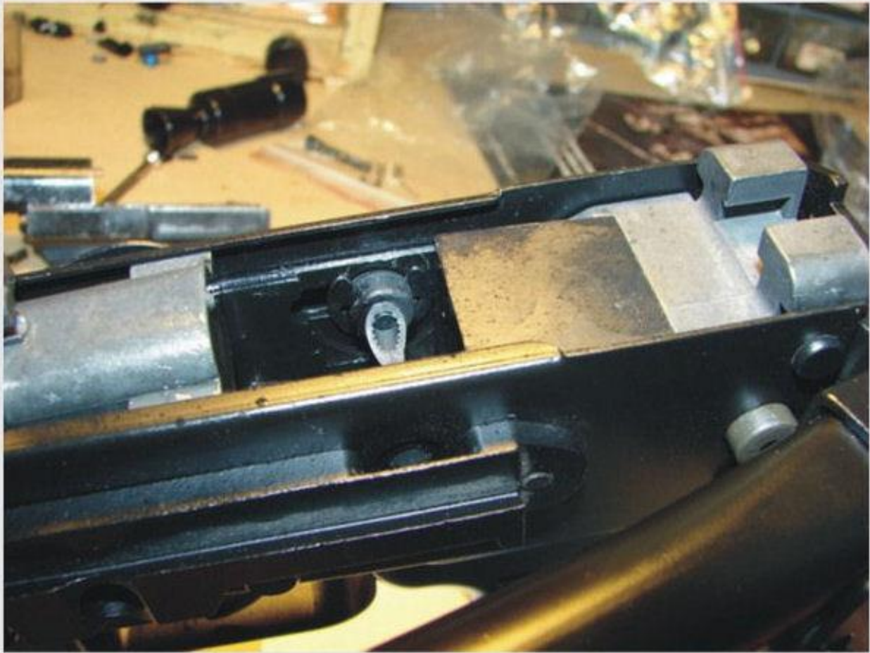
STEP21: The installment of rubber.
