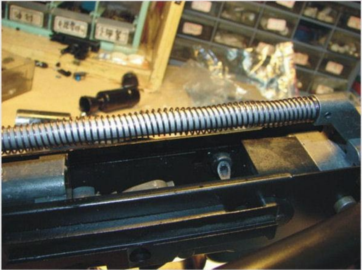
STEP22: The installment of recoil spring set
