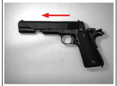
3.REMOVE THE RECOIL SPRING AND SPRING CAP
