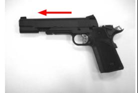
3.REMOVE THE RECOIL SPRING AND SPRING CAP
