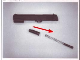
4.REMOVE THE BARREL BUSH AND BARREL
