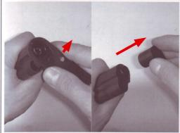
USE WRENCH TO ROTATE THE BARREL BUSH AND REMOVE
